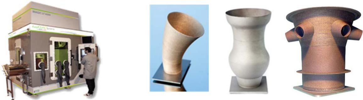
Fig. 17. (a) The machine MAGIC with its inert gas enclosure; (b) Samples manufactured in continuous 5 axis configuration.
