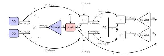
Fig. 4. Composition of mSign (the blue gadgets will be proved d-NIo, the white ones will be proved d-NI and the red one won't be protected)
