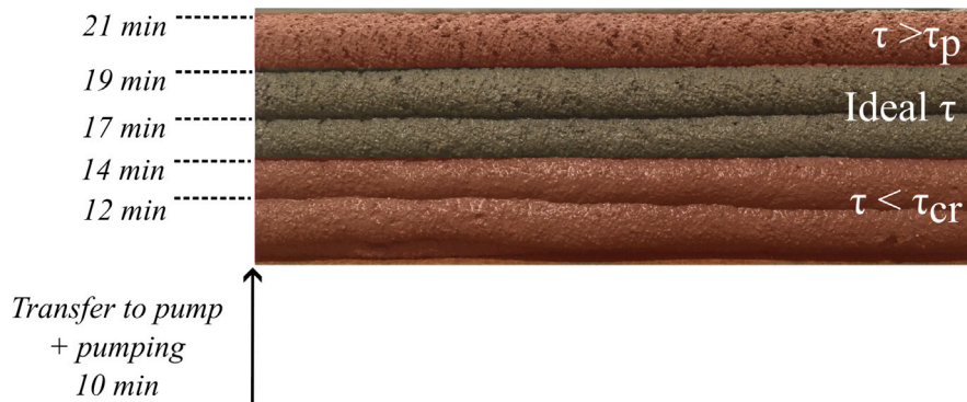
Fig. 3. Resulting print using an initial mixture: the decreasing plastic deformation at deposition, from \tau < \tau_{cr} (in red) to \tau > \tau_p (in red) illustrates the structuration rate. (For interpretation of the references to color in this figure legend, the reader is referred to the web version of this article.)
