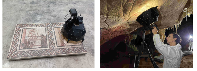
Figure 1. Installation of the RTI dome: (a) on the Seasons mosaic at Saint-Romain-en-Gal (Rhône, France); (b) in front of a painted wall in the prehistoric Chauvet cave (Ardèche, France).
