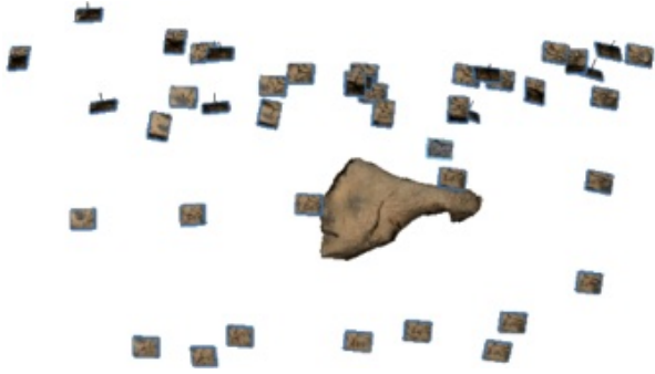
Figure 5. Multi-view acquisition of the “Mask”: camera poses were estimated by structure-from-motion from around twenty photographs taken under constant lighting.
