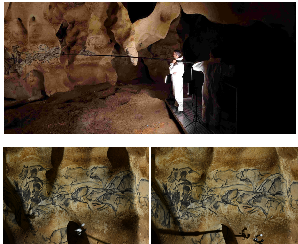
Figure 3. Calibrated PS used in the Chauvet cave (Ardèche, France). Top: the calibration sphere is held at arm’s length at the end of a pole, as it is impossible to get closer than six meters to certain walls. Bottom left: an exposure time that was too long, even though it was well suited to the lighting conditions, rendered the image of the sphere blurred and therefore unusable. Bottom right: the image of the sphere becomes clearer after reducing the exposure time and increasing the aperture of the lens, but this is at the expense of depth of field. Another problem: the pole and the sphere cast shadows on the wall.
