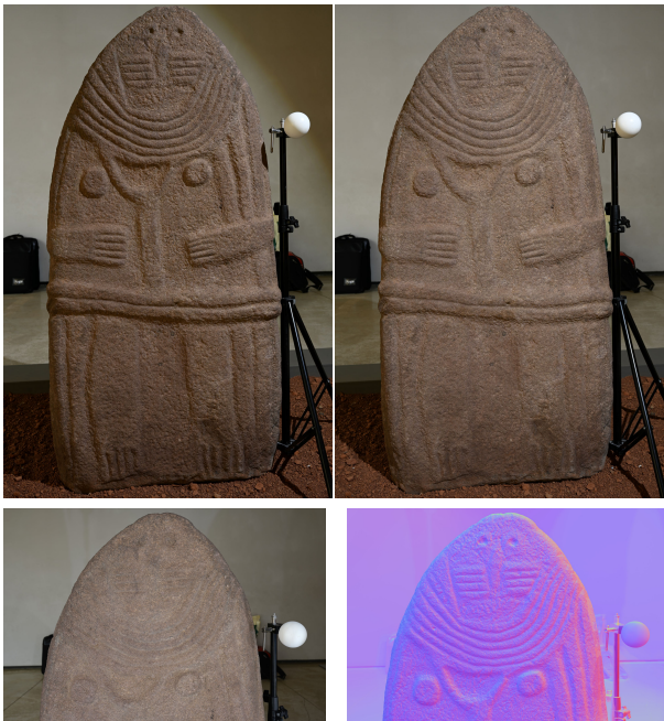
Figure 2. PS applied to the “Dame de Saint-Sernin” statue-menhir (Musée Fenaille, Rodez). Top line: two photographs taken under two different lighting conditions. The white sphere is used to calibrate the lighting. Bottom line: albedo map and normal field estimated from around twenty images. As expected, the estimated albedo of the white sphere is free of shading effects.
