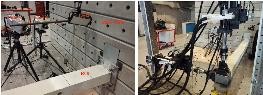
Fig. 6 Experimental setup. (left) Stereovision system. (right) Tested RCC with two actuators
