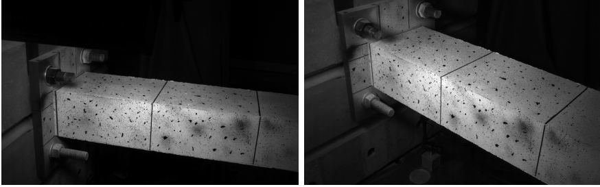
Fig. 7 Reference images captured by the two high-speed cameras. Left and right are respectively cameras 1 and 2
