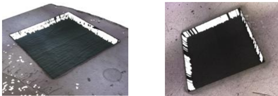
Figure 3. Ablated craters 1 \times 1 \text{ mm}^2 in enamel (left) and dentin (right) imaged with OM.
