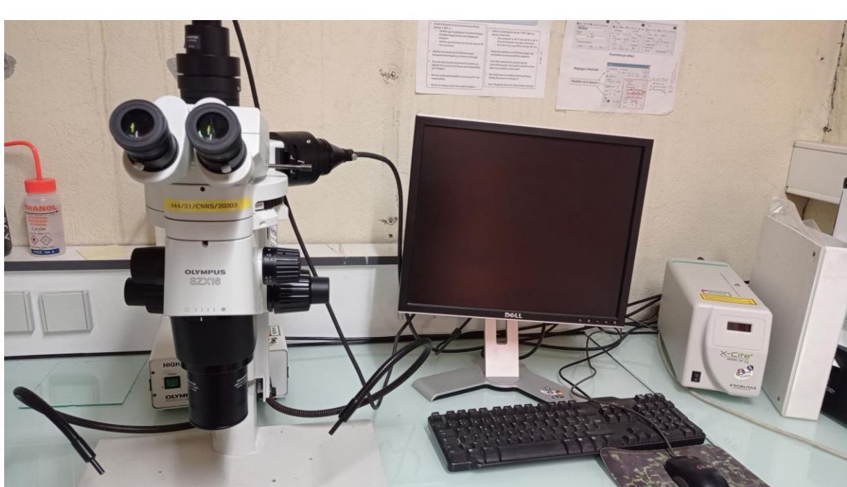
GFP SZX12 binocular magnifier (microscope objectives X7 to X90-ocular X10)
