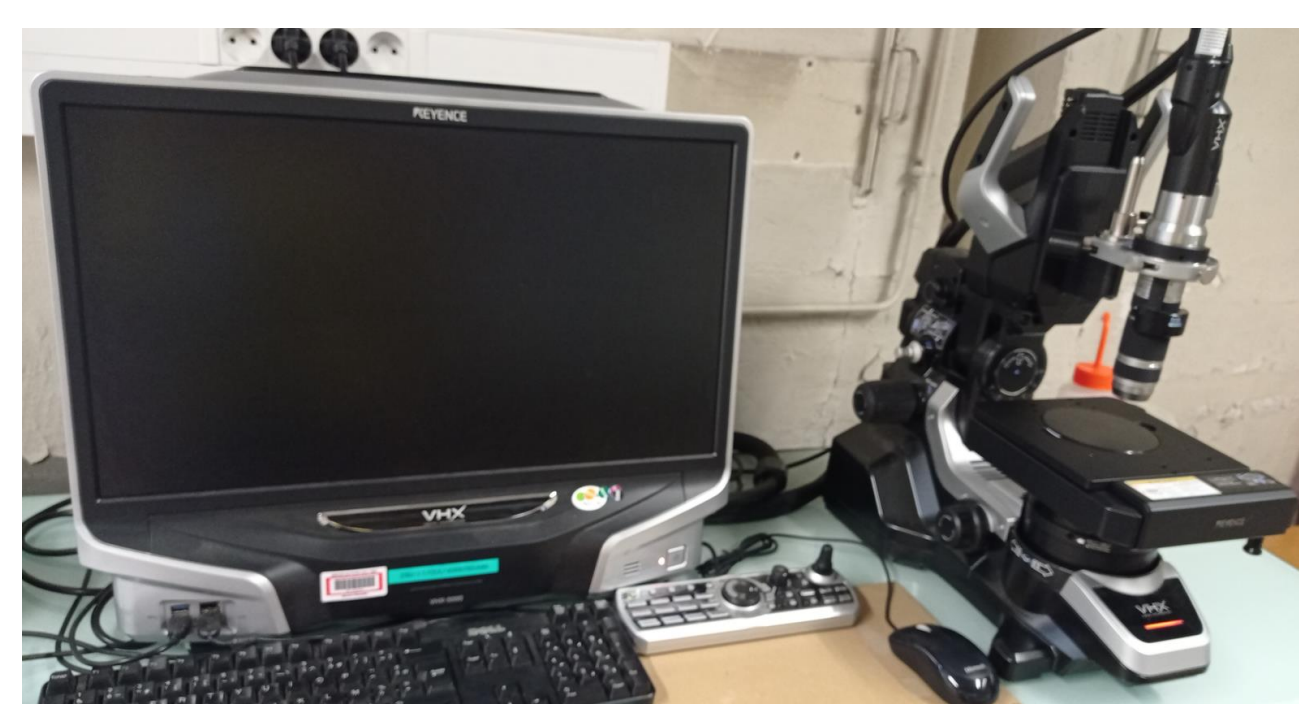
Keyence VHX-5000 3D digital microscope (microscope objectives X20 to X200 and X100 to X1000)
