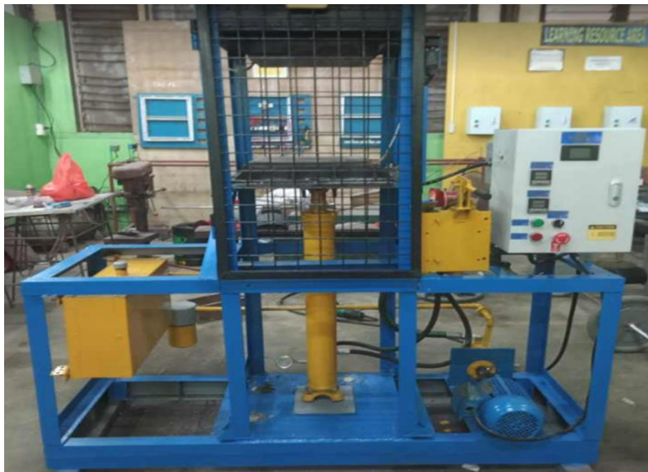
Figure 8. The fabricated hot-pressing device
