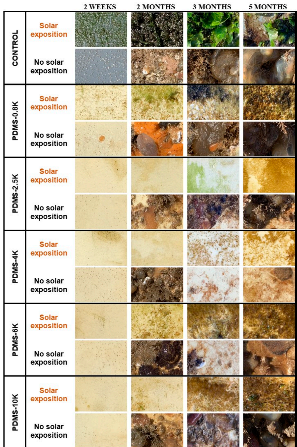
Figure 7. Macrofouling development observed on PDMS-based coatings (4 cm × 3 cm).
