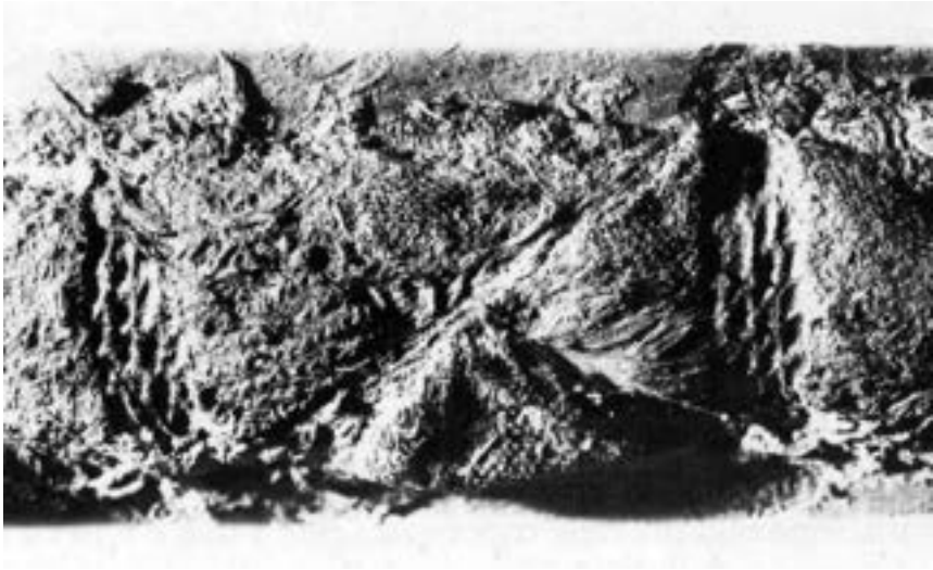
Figure 8: Detail view of the sewing system of the Comacchio shipwreck. Credit/source: from Berti 1990, p. 30, fig. 4.
