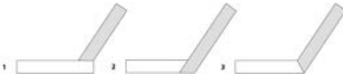
Figure 23: Schema of the different arrangements of bottom-based barges without carved bilge planks: 1. Projecting bottom plank; 2. Internally-set bottom plank; 3. Chamfered bottom plank. Credit/source: drawing by G. Boetto, CNRS/CCJ.
