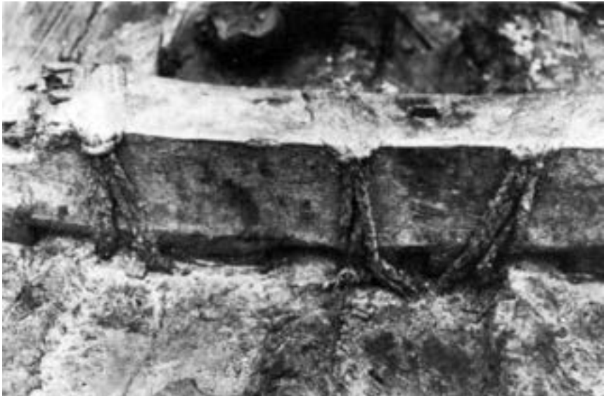
Figure 9: Detail view of the external lashing attaching the frames to the planking of the Comacchio shipwreck. Credit/source: from Berti 1990, p. 31, fig. 10.
