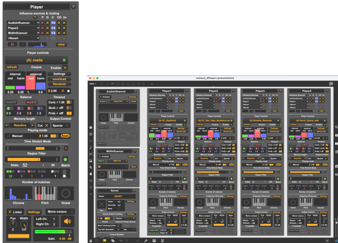
Figure 6. Somax2 usual GUI (right) and a player detailed (left). Inside a player, from top to bottom : source influence routing interface, streamview layers balance for self and external influence, statistical model variable memory length, matches visualisation, output influence interface, rendering interface.
