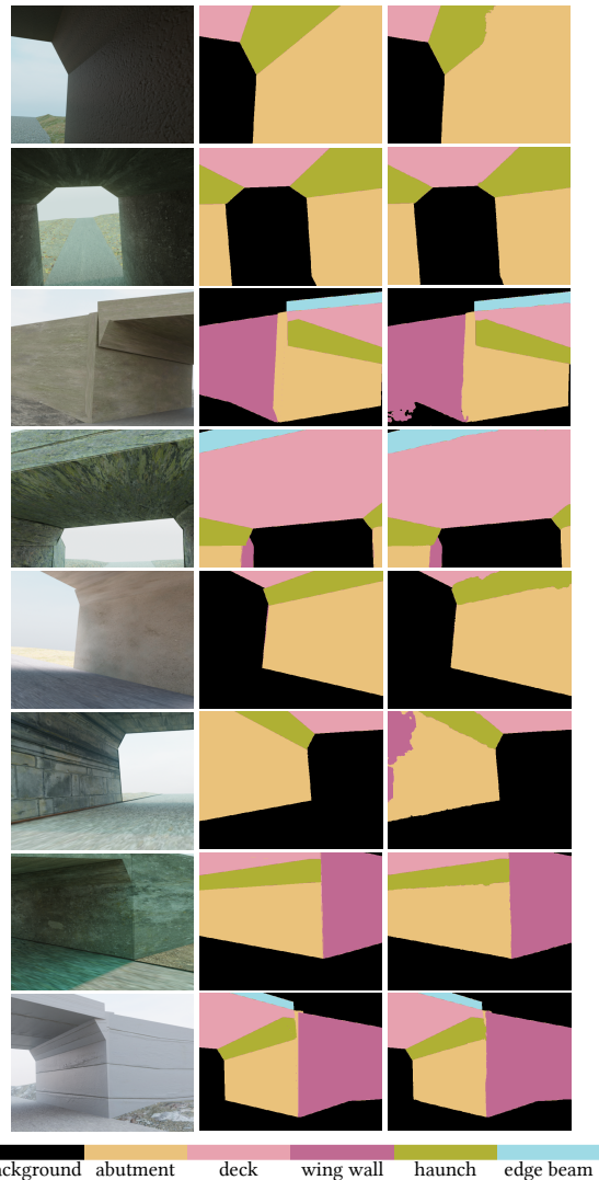
Fig. 10: Qualitative results on synthetic images. The prediction model is a Unet with an Imagenet pretrained MobileNetV2 as backbone, trained exclusively on synthetic data . Left: Image. Middle: Ground truth masks. Right: Network predictions.
