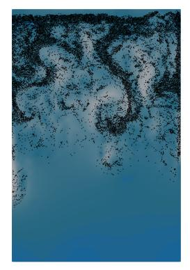
property. Injecting water at the bottom of a deposit suspends grains in the fluid. This process can be repeated indefinitely to artificially create successive settling of grains. Starting from an unsorted granular matrix, it is possible to sort the grains to isolate grains having the desired property.
