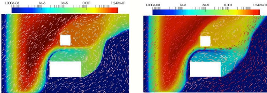
FIGURE 2 – Concentration solution (logarithmic scale) over velocity field. Left : with  $\mathbf{p}_v = 0.1 \frac{m}{s}$  and  $\mathbf{p}_s = 1 \times 10^{-3} \frac{mg}{m^3}$ . Right : with  $\mathbf{p}_v = 1.3 \frac{m}{s}$  and  $\mathbf{p}_s = 1 \times 10^{-2} \frac{mg}{m^3}$ .
