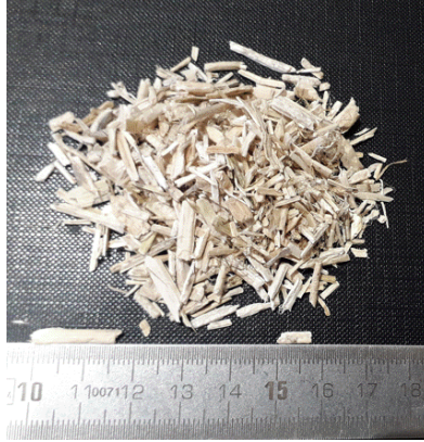
Fig 1. Hemp shiv particle used for this study (size ranging from 2 to 14 mm)
