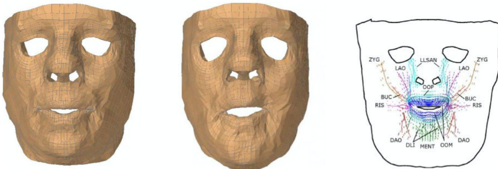
Figure 3: Face FE modeling symmetric (left) and asymmetric(middle) and facial muscles network (right).
