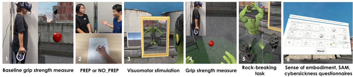
Fig. 3. Overview of the experiment’s procedure. 1) Baseline grip strength (maximum and goal-oriented) is measured using a hand dynamometer. 2) Condition PREP or NO_PREP is applied. 3) The participant is immersed in VR and goes through visuomotor stimulation. 4) The grip strength is re-measured. 5) The participant proceeds to the rock-breaking task. 6) Finally, they complete an SoE, SAM, and cybersickness questionnaire before exiting VR.
