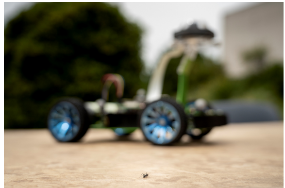
Fig. 1 Biological inspiration for robotic navigation. An ant in the foreground symbolizes nature’s efficient navigational strategies, while the Antcar robot in the background integrates these principles into a neuromorphic system. The blurred image captures only the large masses of the environment, similar to the low-pass spatial filter in the ant’s visual system, which retains these large features even when objects obstruct the view between the robot and the building. ©Tifenn Ripoll - VOST Collectif / Institut Carnot STAR.
