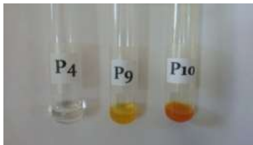
Figure 2. 2.5 mol% vinyl-PDMS oil P4 (left), Fluorescein containing-PDMS oil P9 (middle) and P10 (right).
