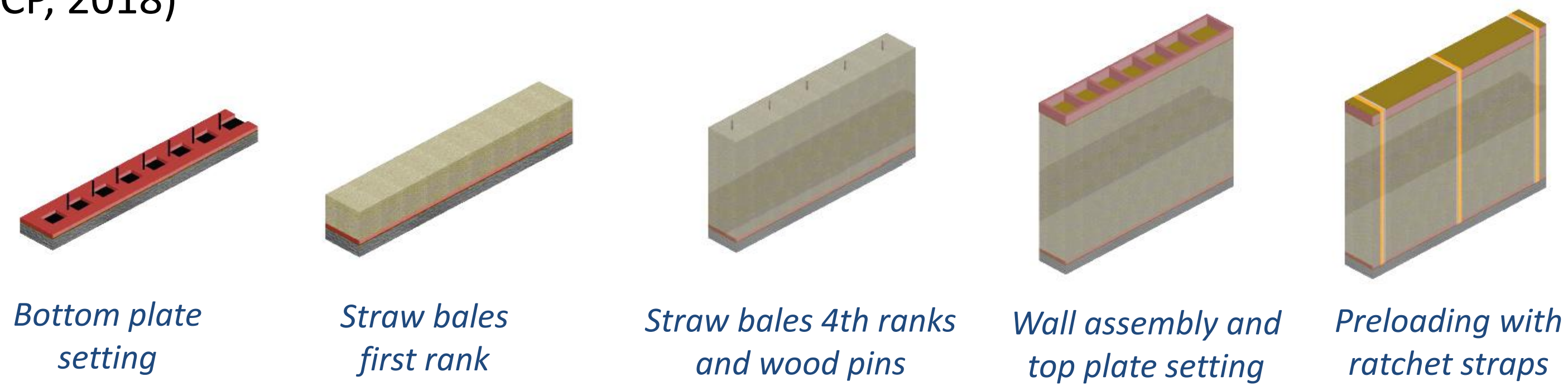
Figure 1 – Wall assembly using Nebraska technique (Source : J. Lossignol, 2021)
