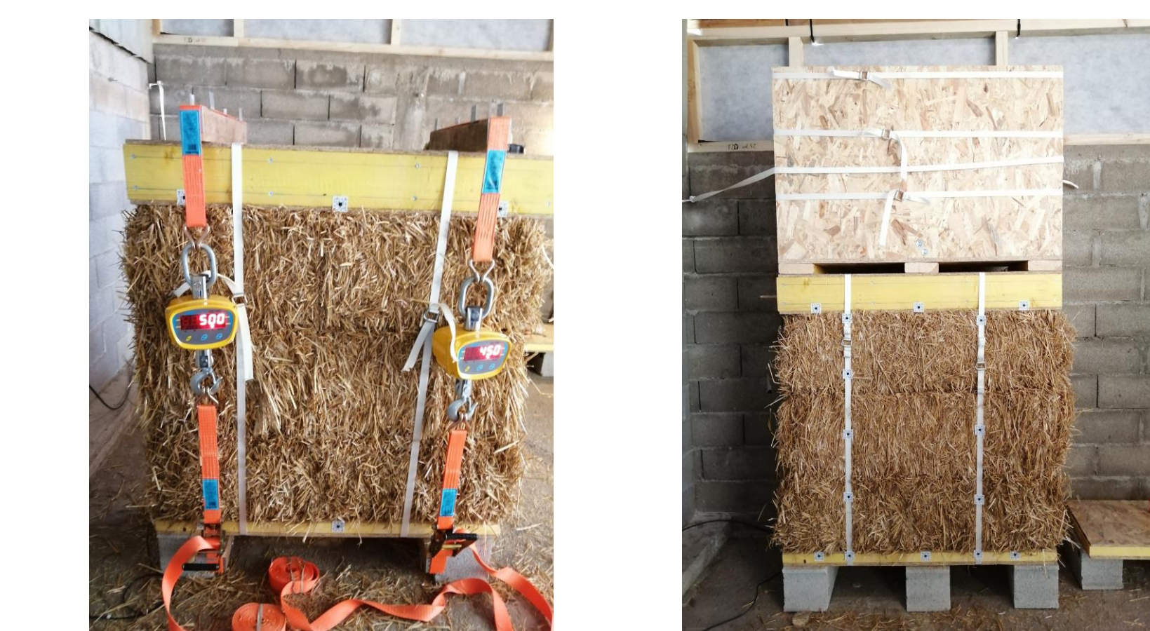
Figure 6 – Test setup (Source : Photo library - J. Lossignol, 2021)
