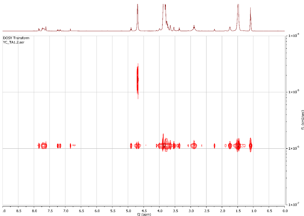
Figure 9. DOSY map for a solution of C_{12}E_{23} 0.03 \text{ mol}\cdot\text{L}^{-1} , OPA 0.03 \text{ mol}\cdot\text{L}^{-1} , mercaptoethanol 0.03 \text{ mol}\cdot\text{L}^{-1} and HA 0.01 \text{ mol}\cdot\text{L}^{-1} in the Roth medium.
