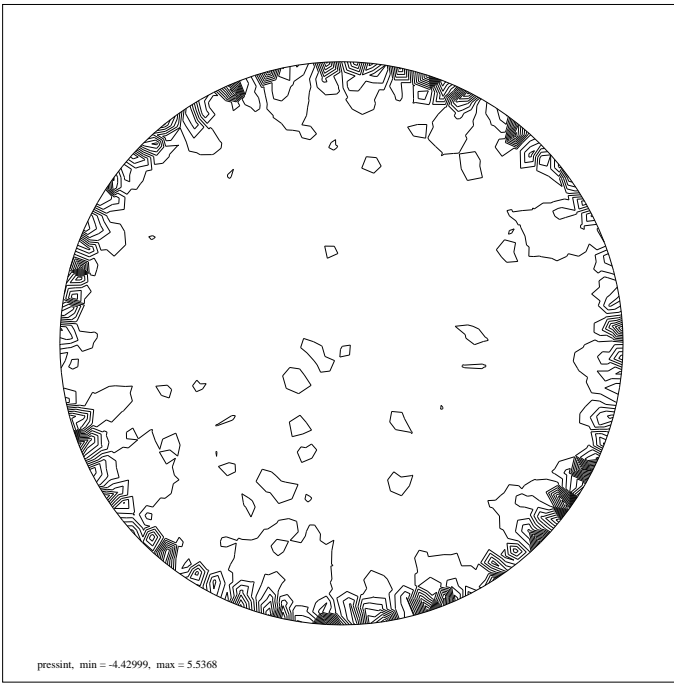
Fig. 25. Numerical pressure isovalues - Test proposed by Ruas on an unstructured mesh - Expected pressure : 0 - Computed extrema : -17.5 to 12.8 !
