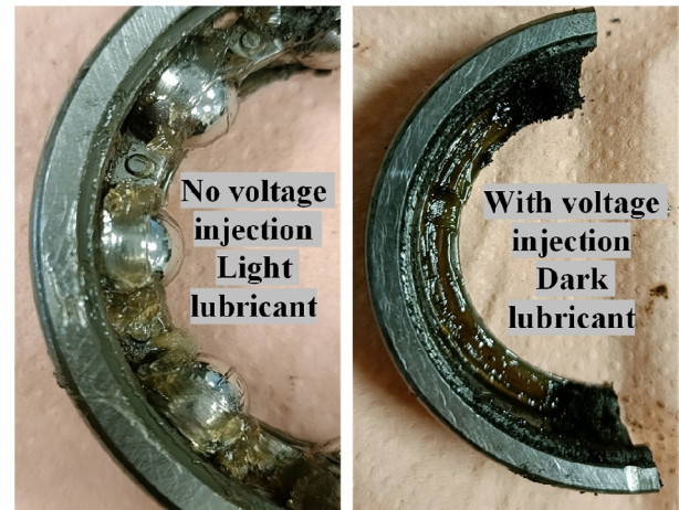
FIGURE 10 Lubricant chemical change due to electrical wear.
