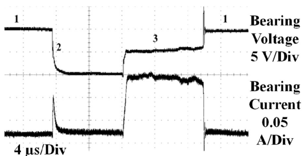
FIGURE 5 Different lubricant behaviours: (1) insulating behaviour (full film), (2) electrical discharge machining, and (3) conducting behaviour during 'short conduction'.
