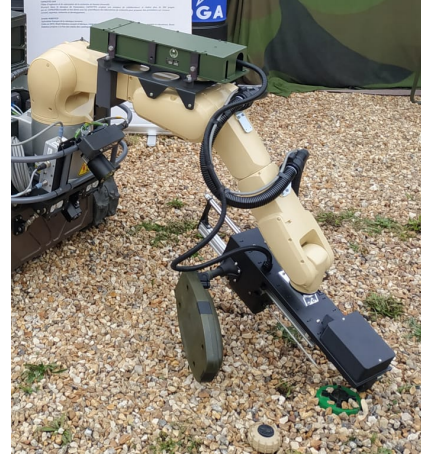
Fig. 1: In-house development of an autonomous probing system aimed at detecting, localizing and classifying underground objects.
