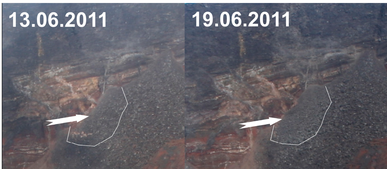
Figure 10. The white arrows show visually detectable surface changes (DoDs) in rock zone II between 13 June 2011 and 19 June 2011.
