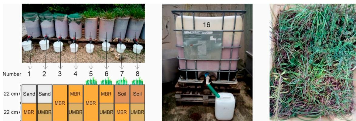
**Figure 2.** Lysimeters experimental setup. Left: 40-L lysimeters, view and diagram of filling and revegetation; center and right: 700-L lysimeter, shown from the side and from above, respectively.
