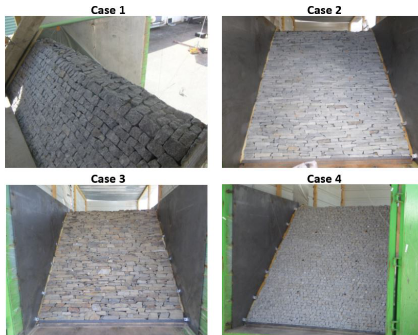
FIGURE 3 Dry-stone pitching of the four physical models in PEDRA experimental campaign
