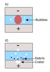
Fig. 1 Machining steps by µEDM.
