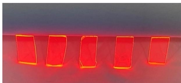
Figure 1. Strong visible red emission of Eu-doped films in PMMA under UV light.
