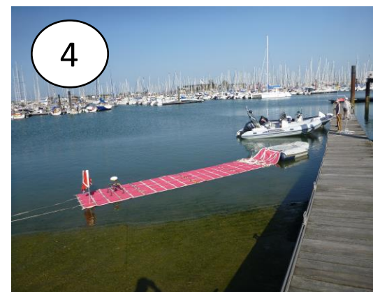
GNSS carpet (CalNaGeo) towed by Tidalou boat
