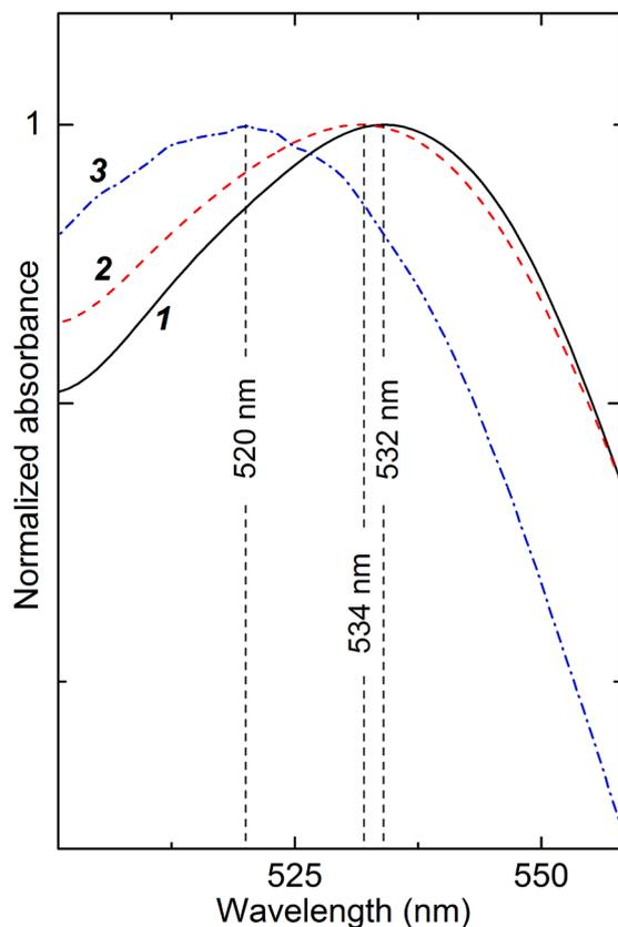
Fig. 4. Normalized absorption of the mesoporous TiO<sub>2</sub> film with neat N719 dye (1) and after sequential co-adsorption with PVBA (2) and P4VP (3).
