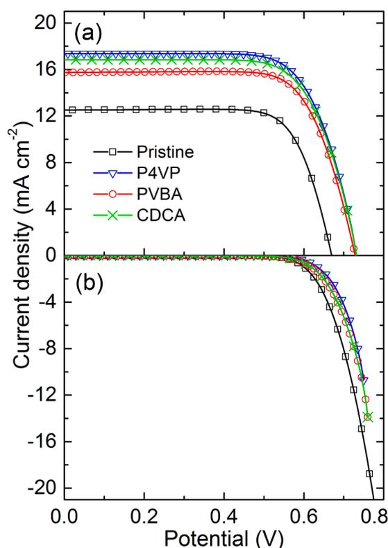
Fig. 5. *I*-*V* curves under 1- Sun equivalent (a) and in the dark (b) of the DSSCs with pristine TiO<sub>2</sub>/dye photoanode (squares); after co-adsorption of P4VP (triangles), PVBA (circles) or CDCA (crosses).
