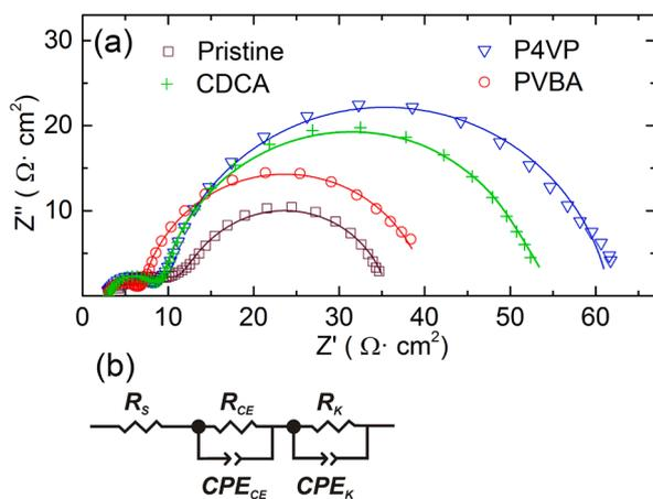
**Fig. 9.** Nyquist diagrams for DSSCs with pristine  $TiO_2$ /N719 photoanode (squares); passivated with P4VP (triangles), PVBA (circles) or CDCA (crosses) (a). Solid lines show the fittings to the equivalent circuit model (b).
