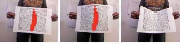
Fig. 2: Two images with ill-conditioned data shown in red. The estimated normals are highly erroneous in this region. To compute the normals in this region, third image is considered.
