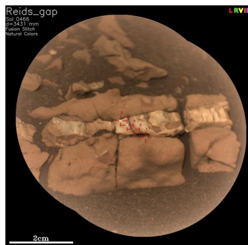
Figure 4: Calcium-sulfate veins such as the target Reids_gap sampled on sol 466 at the delta front can be identified by their high S spectral unmixing score together with high Ca.
