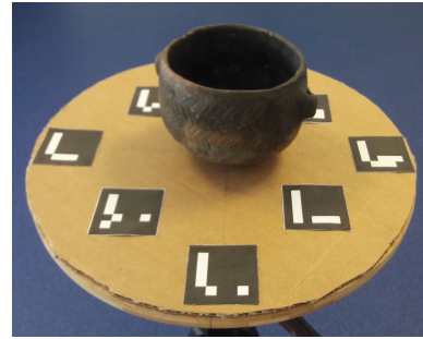
Figure 5: Augmented Reality markers used to track the participants' position relative to the object
