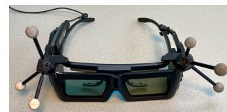
Figure 3: Eye-tracking glasses and stereoscopic glasses attached together with a 3D-printed clip
