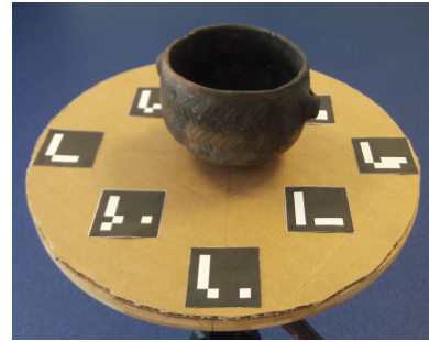
Figure 5: Augmented Reality markers used to track the participants' position relative to the object
