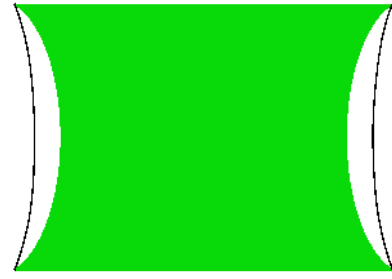
(a) Model fitted to Uniaxial test only. Ogden model with \mu_1 = 4.82\text{E-}2 MPa, \alpha_1 = 3.91 , \mu_2 = 2.8 MPa, \alpha_2 = 0.27 has been used (Corre, 2018).
