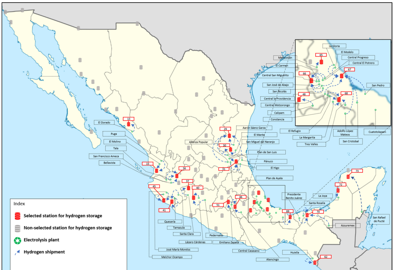
Figure 8. HSC configuration obtained by GWP O.F. optimization.
