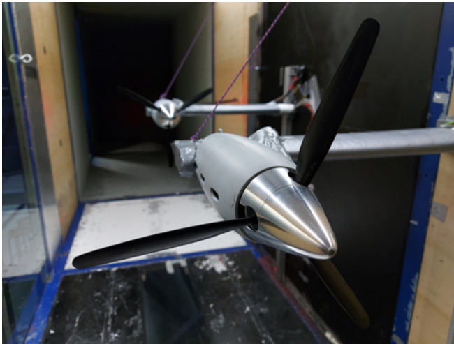
Figure 3. Set up of tandem propellers in cruise flight conditions at the S. De Ponte wind tunnel.
