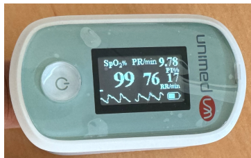
FIGURE 9: Pulse oximeter used for RR and RH reference
