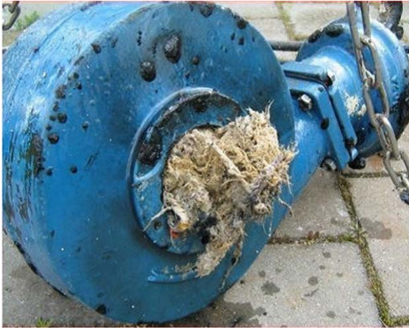
Figure 5.48 Clogged pump. (Source: Deltares).
