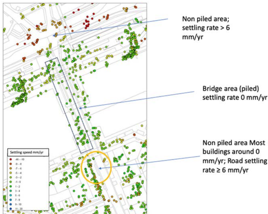
Figure 5.55 Observed subsidence of the soil, the blue line indicates the location of the pressure main, the red area indicates the location of the incident, the coloured dots indicate the observed subsidence rate of the soil (red = between -46 and -10 mm/year, the green dots between -3 and +4 mm/year the blue dots between +11 and +20 mm/year) As can be seen the differences in subsidence rate in the indicated area are quite high: up to 50 mm/year).
