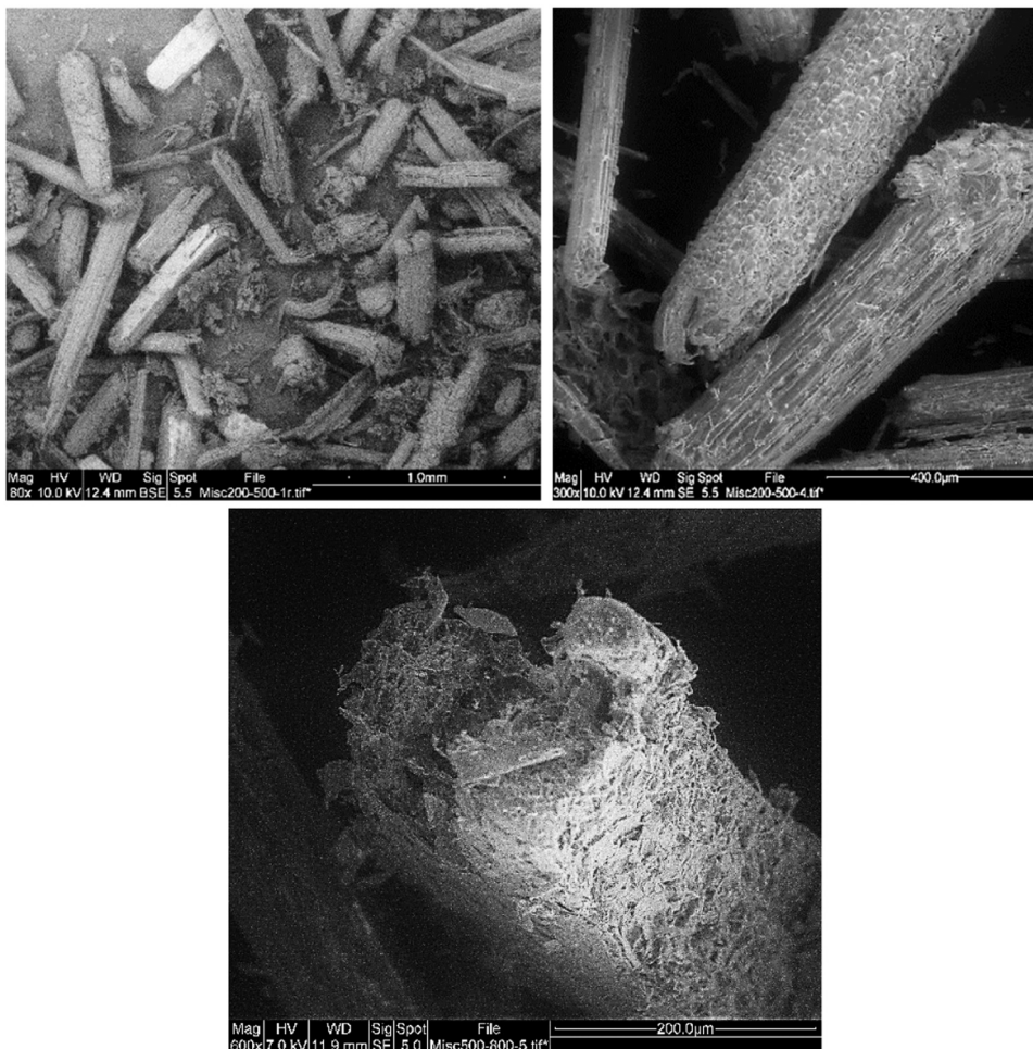
Fig. 1. Scanning Electron Microscopy (SEM) images of the micronized miscanthus fibers at different magnifications.
