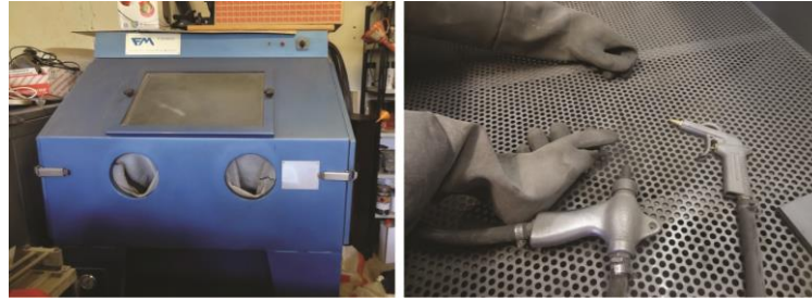
Figure 4: Closed-circuit sandblasting machine, external view on the left and internal view on the right.
