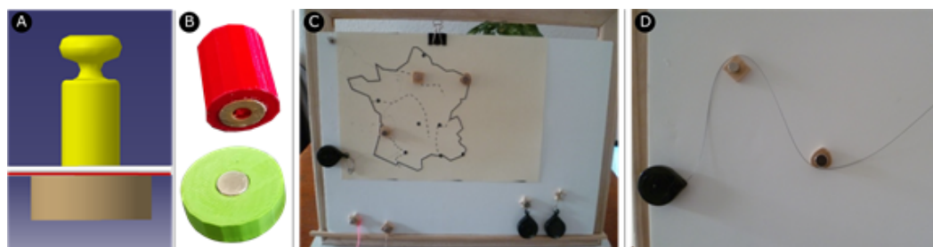
Figure 1. (A) The objects are composed of two parts: one is placed above the surface (accessible to the user); the other is placed below the surface and is tracked by a camera. (B) Both parts are magnetically linked to each other to ensure stability. (C) First low-fidelity prototype with tangible objects on top of a raised-line map of France. The camera is placed behind the vertical board. Different shapes trigger different feedback. (D) Using retractable reels to create tangible line graphs.
