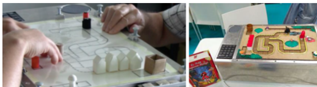
Figure 8. Evolution between the first versions and latest prototypes of the games. (Left) Use of swell paper with black and white colors only and paper/cardboard objects. (Right) Use of a laser-cut wooden board with customized 3D-printed objects and colored stickers.
