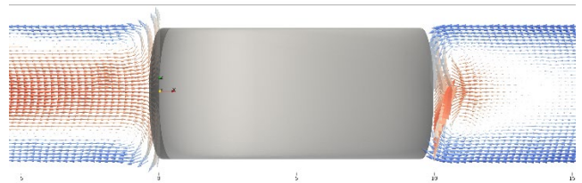
Figure 2: Description of the 3D velocity field around the large bubble ( Ar = 4630 , Bo = 30 ) by tomo-PTV technique. Transverse view of the liquid velocity vectors in front of the bubble and in its near wake in the central plane (the height of the figure is w = 1 \text{ mm} . The bubble is represented arbitrarily in grey color. Reference frame is the one of the bubble. The bubble front is on the right side.).
