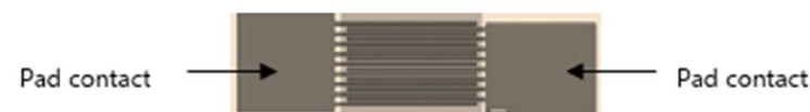
Figure 1. Electrical microdevice design used for sensing performance evaluation with 16 Pt electrodes of 100 \mu\text{m} width. The distance between each electrode is 50 \mu\text{m} .
