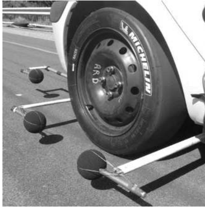
Fig. 13. Close proximity noise measurement system (only the two side microphones have been used for the experiments).
