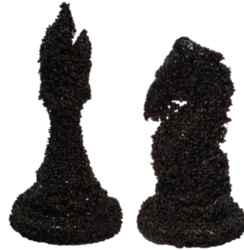
Fig 4: SLM-made bishop and knight chess pieces, both with a 1 cm base diameter
