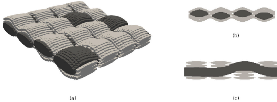
Fig. 6. (a) Geometry used to represent the unit cell of the fabric warp tows are dark gray and weft tows are light gray. (b) Slice along the weft tows. (c) Slice along the warp tows.
