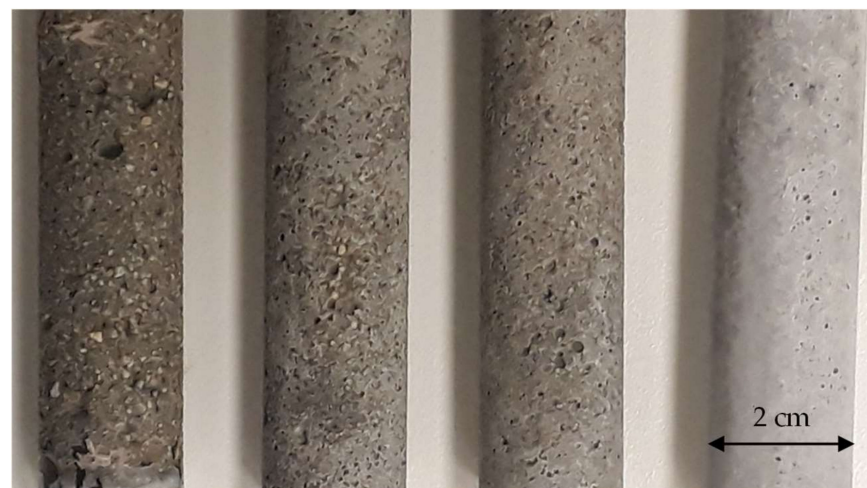
Figure 4. Samples after the immersion period (from left to right: immersed in demineralised water, hard water LSI+0.5-2, soft water LSI-1.0-2, and lime-saturated water).
